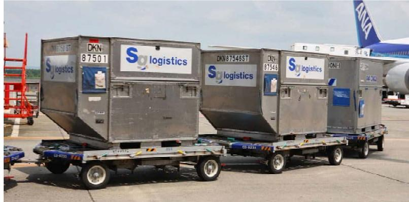
*Fig 3.1: Unit Load Devices*
